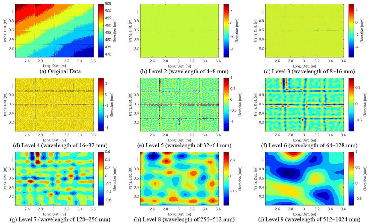
Figure 5. Multiresolution Analysis of Block Pavement
